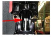
2.4 The two halves are now ready to be put together. You may find it easier to use two people to do this. As you bring the halves together, the first thing that needs to line up is the copper water tube with the plastic tube guide.
